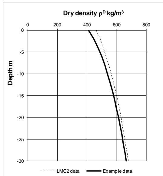
Setting the Reference value, Reference stress and Power law index parameter values in the editor group **Dry density and permeability**, found by clicking on the Tab **Active elements**, determines the relationship between the value of the two properties and effective stress. The relationships used in LDAT are the power law formulations derived by Powrie and Beaven.
